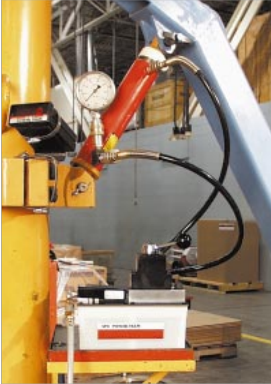
PA6D pump, DG100 digital pressure gauge and 25 ton cylinder used in a test fixture.
