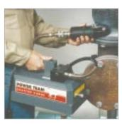
The Quarter Horse pump has a maximum operating pressure of 10,000 psi, which handles a wide variety of hand held hydraulic tools.
