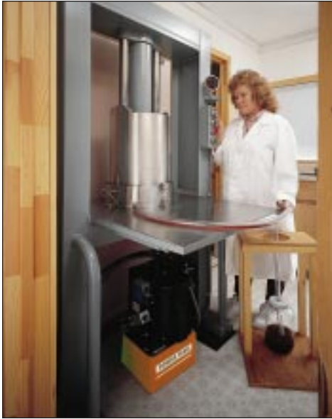
PE21 series pump and RD5513 cylinder used in a special press that produces pharmaceutical-grade extracts for herbal medicines.
