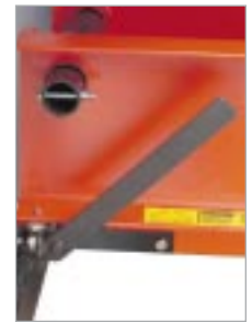
Lever lowers bed for pressing, raises it for rolling.
