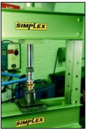
A manufacturer of industrial gear boxes used the Simplex 25 ton press in their production assembly line to press various size bearings on gear assemblies. "We can press up to 100 bearings an hour with the Simplex press. The hydraulics are reliable and easy to use and they keep working day after day."
